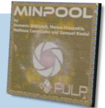
MinPool (2021) 16 cores, 200 MHz TSMC65, 2.4mm x 2.4mm
