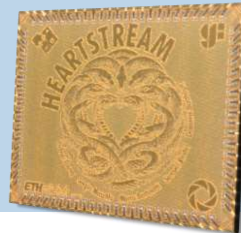
Heartstream (2024) 64 cores, 720 MHz GF12, 2.5mm x 2mm
