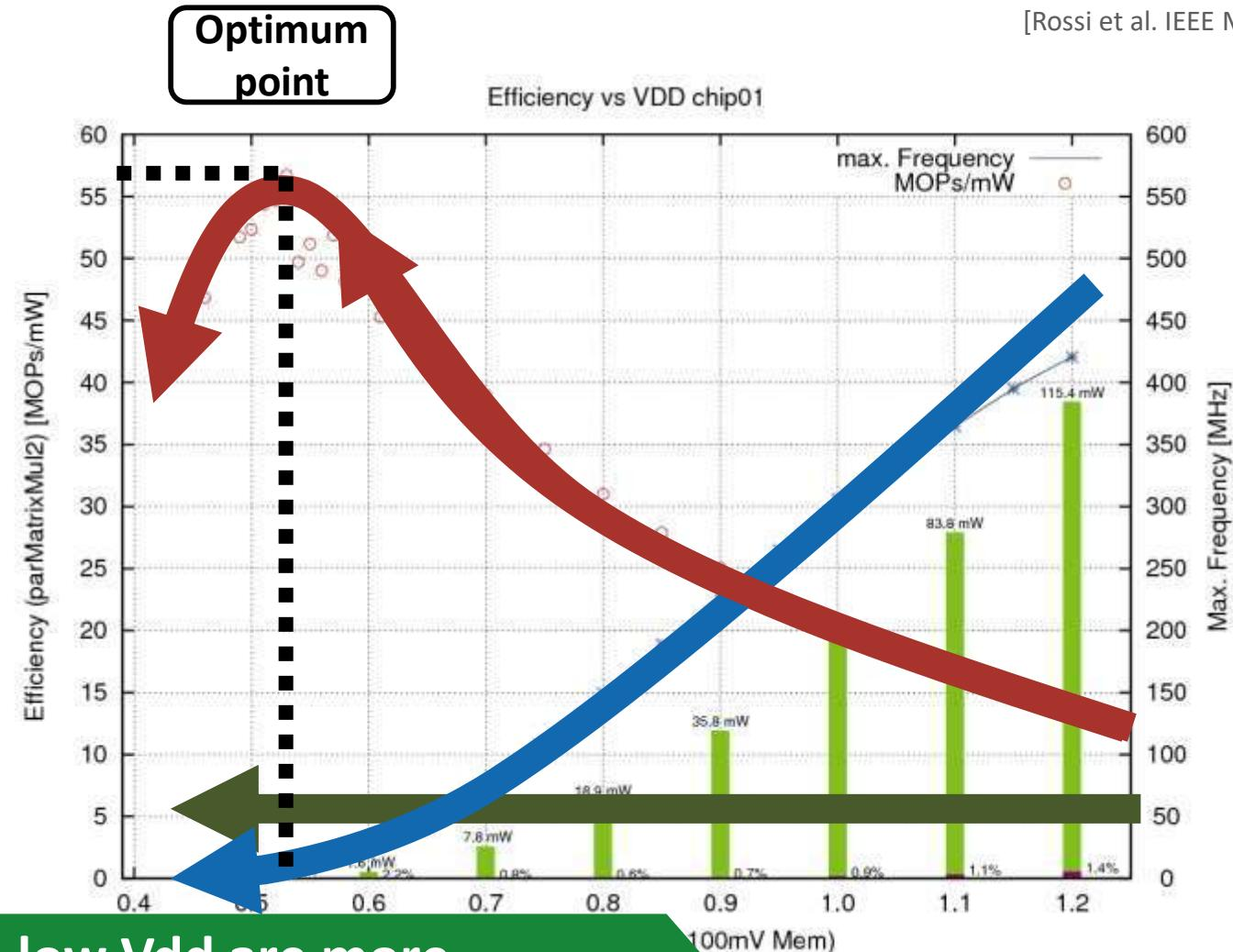
N cores running at moderate f, low Vdd are more energy efficient than a single core at Nxf, high Vdd
