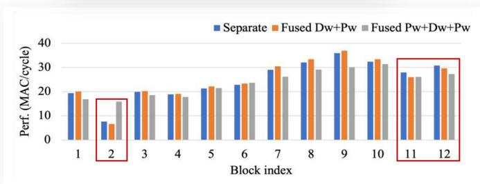
**Result 3:** Achieved 91% and 89% accelerator utilization on MobileNet-V1 and MobileNet-V2 respectively. Speedup of 3.44x over DORY on GAP8 (no acc.).
