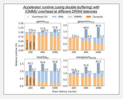
Even on compute bound kernels (GeMM), IO page walking can increase accelerator's runtime by 17.6% under high DRAM latency. Memory bound kernels (GeMV) can face even much larger overheads: 85.6%
