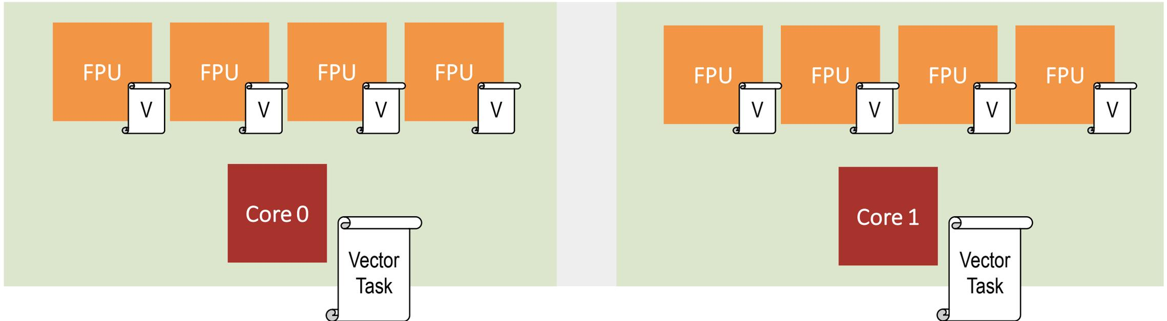
Each core runs a vector task – We can reach 100% FPU utilization!
